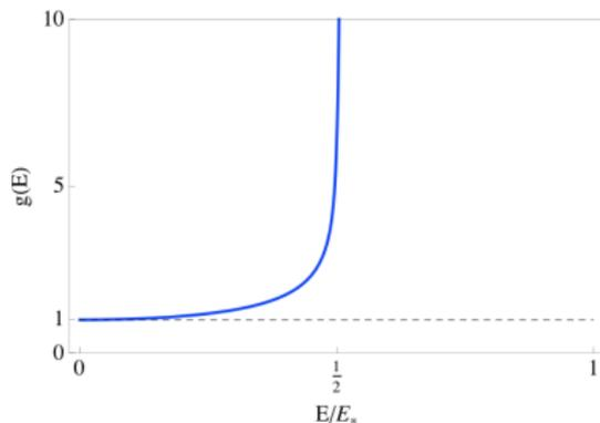
Group velocity:  $v_{\text{gr}} = \beta \sqrt{g(E)}$
